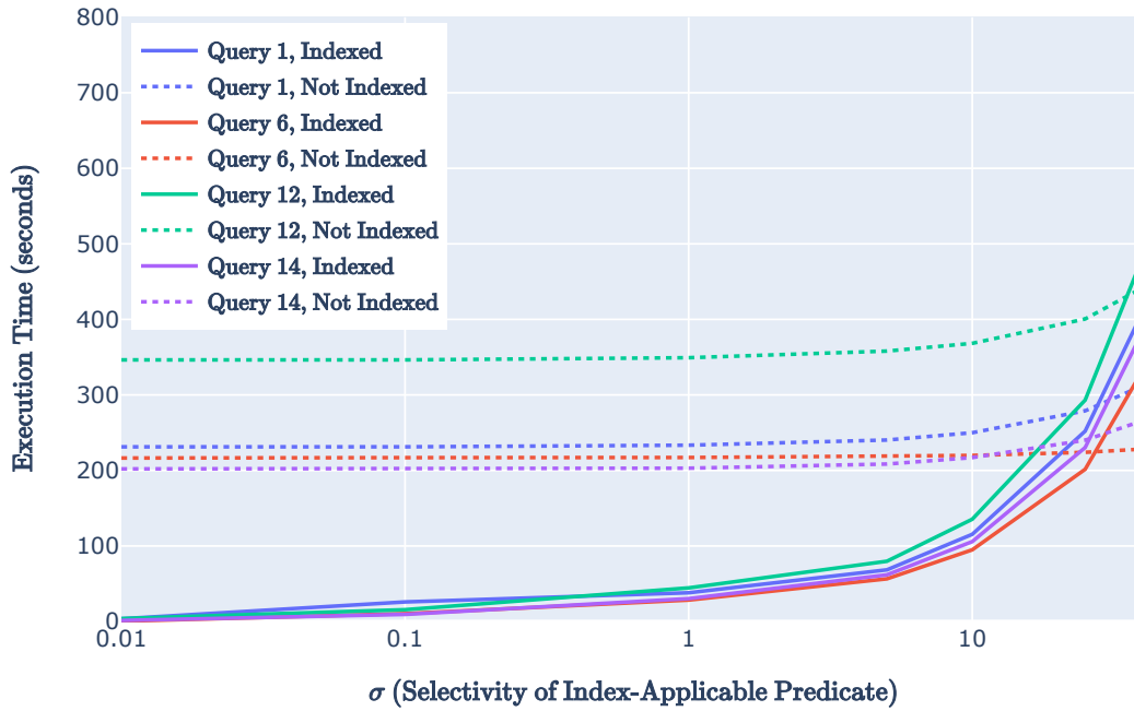
Figure 6.4: Indexed vs. not-indexed query execution times for query set 1.
